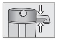
■ Dismantle all the pieces and clean them. To remove the steam spout grip it securely top and bottom as shown and pull it off.
